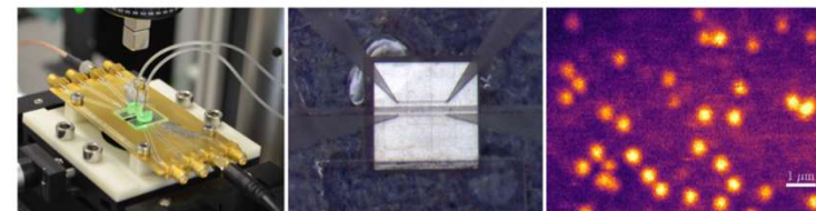
FIG. 15. Confocal imaging of single NVs in a microfluidic device. On the left, a silica glass chip for microfluidic experiments mounted on top of a gold PCB. The chip is illuminated with a green laser. Two needles installed on the inlet and outlet entries lead a flow of the studied fluid through the tubes into the chip. On the center, a microscope image of the 2 \times 2 \text{ mm}^2 CVD-grown diamond installed on top of the microfluidic channels. On the right, an XY scan of single NV centers at a concentration of 10^{11} \text{ cm}^{-2} . The NVs appear distinguishable despite the changes of the refractive index between surfaces.
