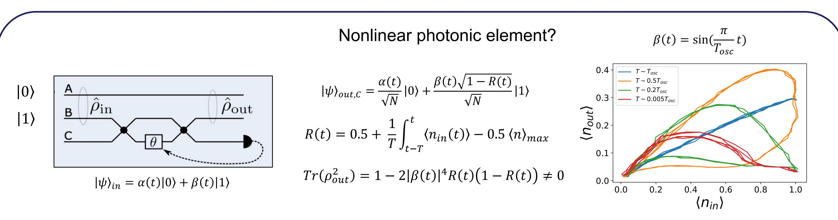
The quantum memristor displays a **nonlinear behaviour** and **short-term memory**, preserving quantum coherence<sup>1</sup>.
