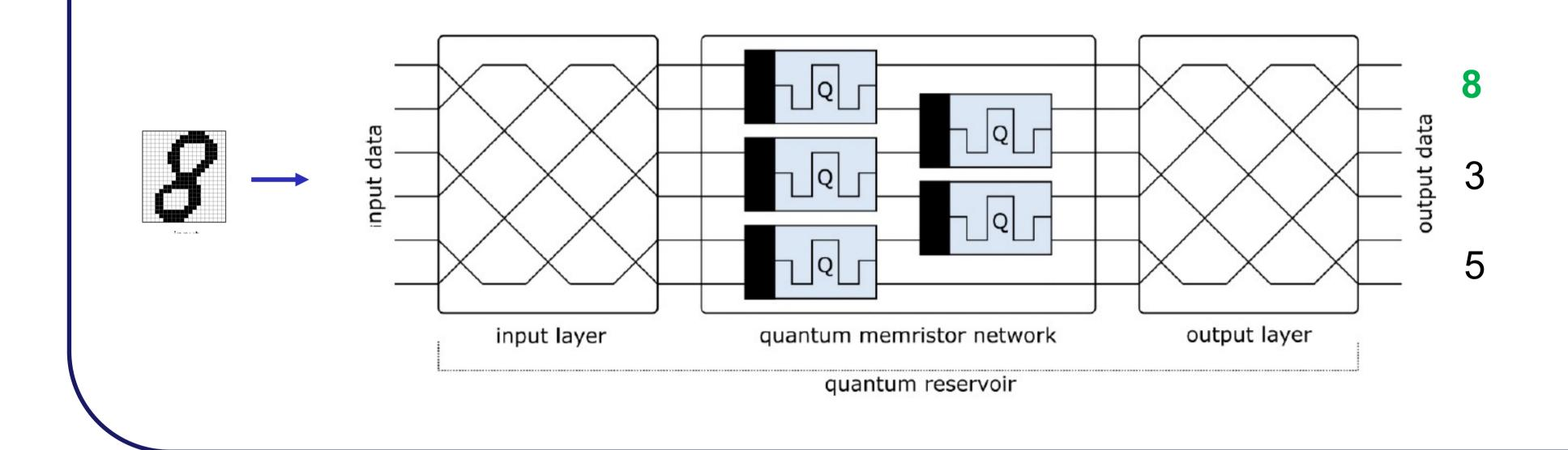
The goal is implementing a quantum neural network, whose nonlinearity is given by quantum memristors. This can be a building block for future quantum neuromorphic architectures.
